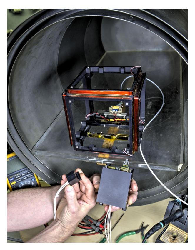
The prototype hybrid magnetometer may fly on a sounding-rocket mission,
