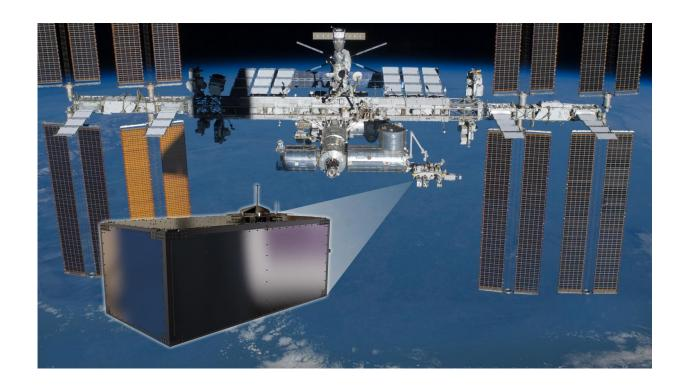
From its new vantage point on the International Space Station's Japanese Experiment Module - Exposed Facility, the Cosmic Ray Energetics and Mass (CREAM) mission, shown in the inset illustration, will study cosmic rays to determine their sources and acceleration mechanisms. Credit: NASA
