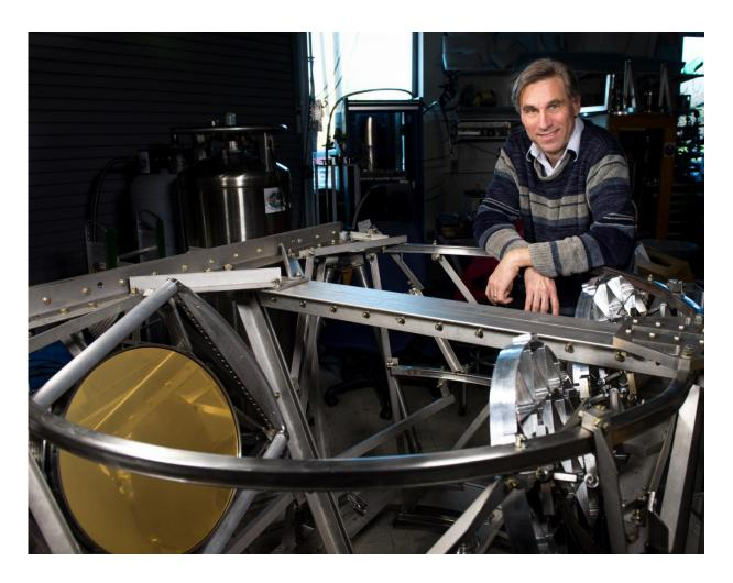
Al Kogut, an astrophysicist at NASA Goddard, poses with one of the millimeterwave telescopes for the Primordial Inflation Polarization Explorer (PIPER) balloon mission. Credit: NASA's Goddard Space Flight Center/Bill Hrybyk
