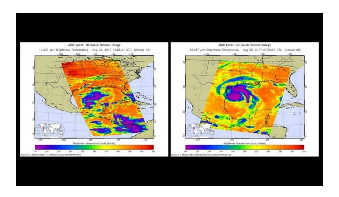
Hurricane Harvey as seen by the AIRS infrared instrument on NASA's Aqua satellite at 3 p.m. CDT on Wednesday, Aug. 23 (left) and at 3 a.m. CDT on Friday, Aug. 25 (right). The darker the color, the colder and higher the clouds and the stronger the thunderstorms. Credit: NASA/JPL-Caltech
