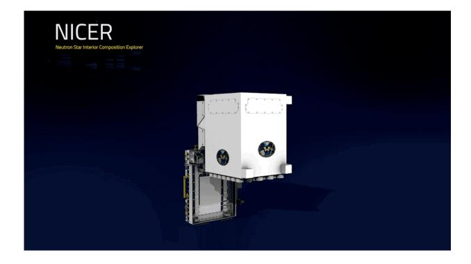
NICER is currently installed on the International Space Station. This turntable animation of the payload calls out the locations of NICER's star tracker camera, electronics, space station attachment mechanism, 56 sunshields, pointing actuators and stow/deploy actuator. Credit: NASA's Goddard Space Flight Center
