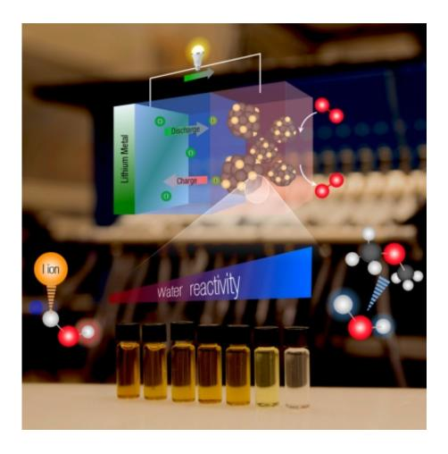
Iodide ions can make water more reactive, altering the reaction pathway during the discharge process. Credit: Massachusetts Institute of Technology
