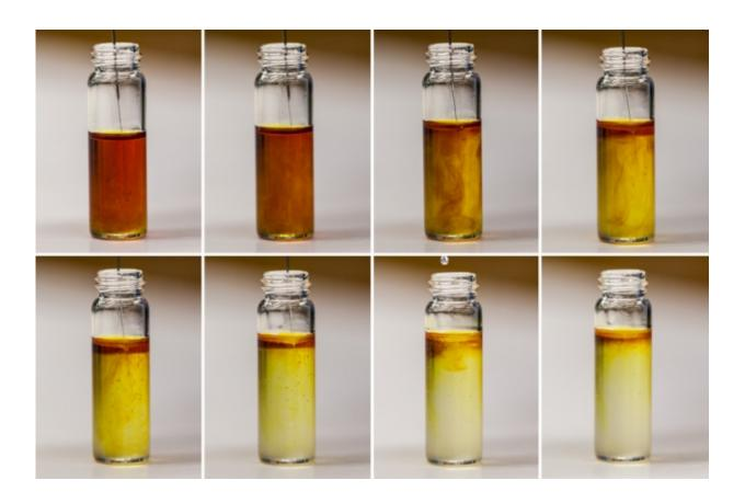
This series of photographs shows the chemical reaction that occurs during the charging of a lithium oxygen battery using lithium iodide as an additive. Credit: Jose-Luis Olivares/MIT
