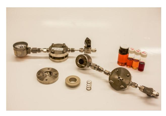
Lithium oxygen battery cell components were used for experiments in the lab. Credit: Massachusetts Institute of Technology
