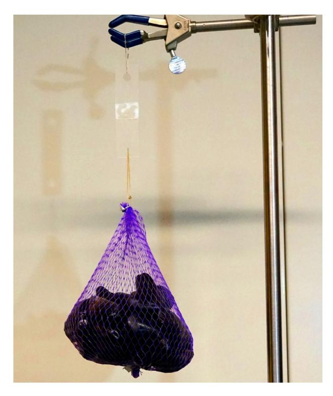
A glue based on a mussel adhesive is strong enough to suspend a bag of shellfish. Credit: Diederik Balkenende
