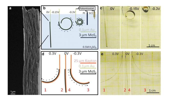
Very thin sheets of molybdenum disulfide (see a), a schematic and photos of working actuators. Credit: Muharrem Acerce/Rutgers University-New Brunswick
