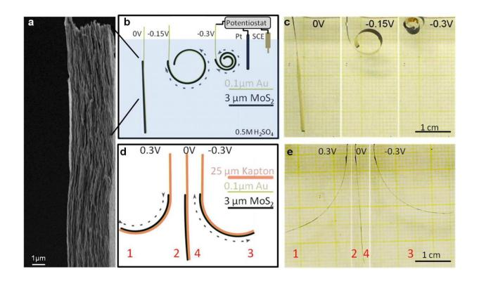
Very thin sheets of molybdenum disulfide (see a), a schematic and photos of working actuators. Credit: Muharrem Acerce/Rutgers University-New Brunswick
