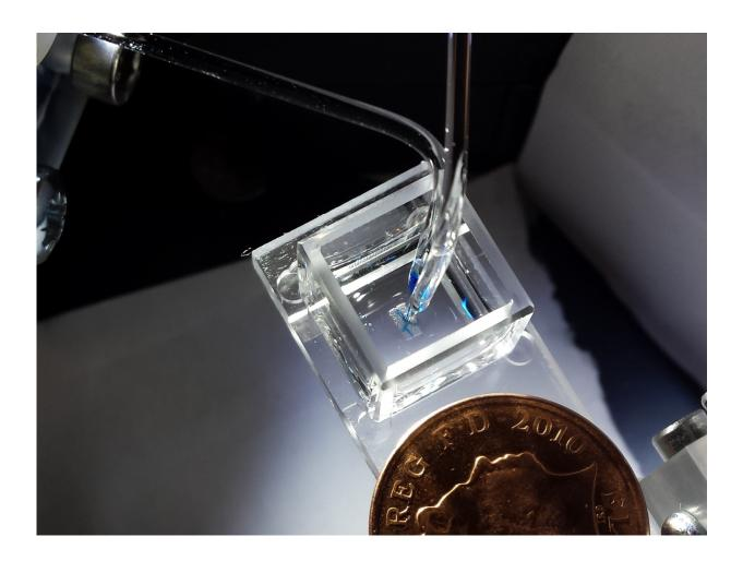
Image of the 3-D droplet bioprinter, developed by the Bayley Research Group at Oxford, producing mm-sized tissues Credit: Sam Olof/ Alexander Graham
