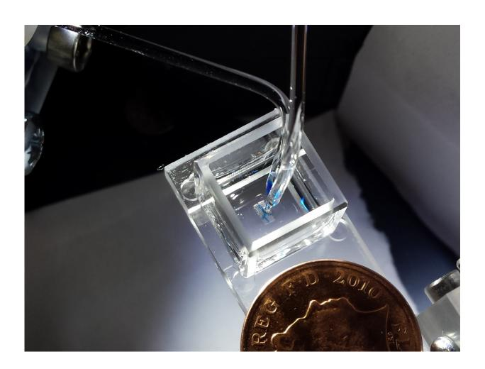
Image of the 3-D droplet bioprinter, developed by the Bayley Research Group at Oxford, producing mm-sized tissues Credit: Sam Olof/ Alexander Graham
