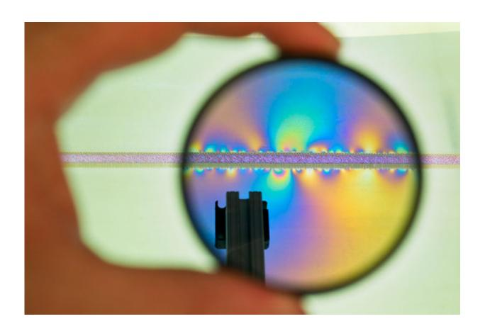
Researchers at Los Alamos National Laboratory have developed a two-dimensional tabletop simulator that models the buildup and release of stress along an artificial fault. In this image, the simulator is viewed through a polarized camera lens, photo-elastic plates reveal discrete points of stress buildup along both sides of the modeled fault as the far (upper) plate is moved laterally along the fault. Credit:Los Alamos National Laboratory
