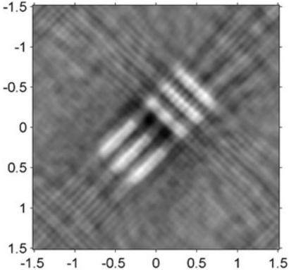
SPIDER's first test used a standard bar pattern used to test optical instruments, result shown here (in millimeters). The team continues to increase the system's resolution from these first, baseline images. Credit: Lockheed Martin
