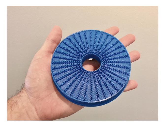
A close-up view of the next phase concept for SPIDER, which would align rows of tiny lenses and its photonic integrated circuits around a circular instrument, still retaining a size around an inch thick. Credit: Lockheed Martin
