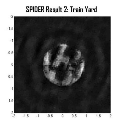
SPIDER's second test used a complex overhead view of a rail yard, result shown here (in millimeters). The team continues to increase the system's resolution from these first, baseline images. Credit: Lockheed Martin
