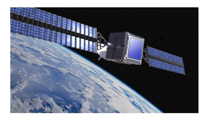
This concept view shows how a SPIDER instrument could be used in orbit on a spacecraft performing multiple missions. Currently, the size of optical payloads makes dual-payload spacecraft difficult and costly. A flat instrument like SPIDER could change all that. Credit: Lockheed Martin
