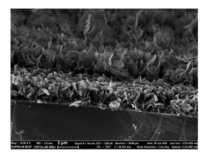
Side view microphotograph of an electrode slice, depicting the structure of a nanowall/silicon/nanowall. Credit: Victor Krivchenko
