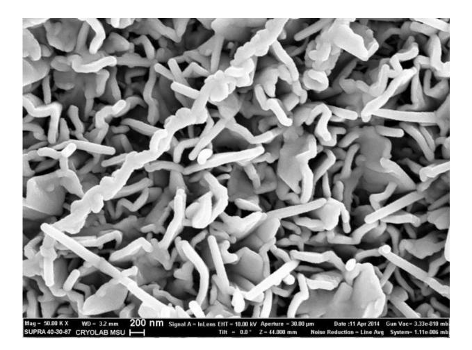
Top view microphotograph of silicon (above) and germanium (below) films on the surface of carbon nanowalls. Credit: Victor Krivchenko
