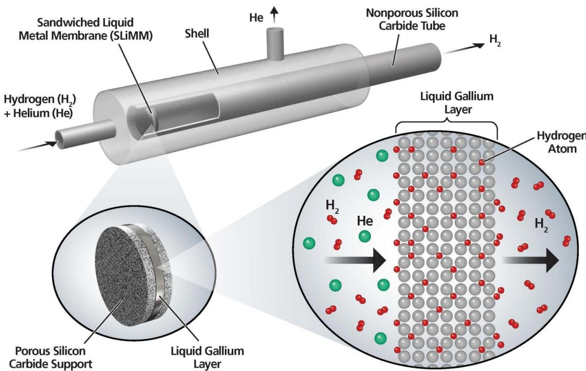
Researchers at Worcester Polytechnic Institute (WPI) tested a prototype sandwiched liquid-metal membrane with this laboratory set-up. The membrane, a thin layer of gallium sandwiched between porous ceramic supports, selectively separated hydrogen from a mixed-gas stream more efficiently than a comparable palladium membrane. Credit: Worcester Polytechnic Institute (WPI)/Curtis Sayers
