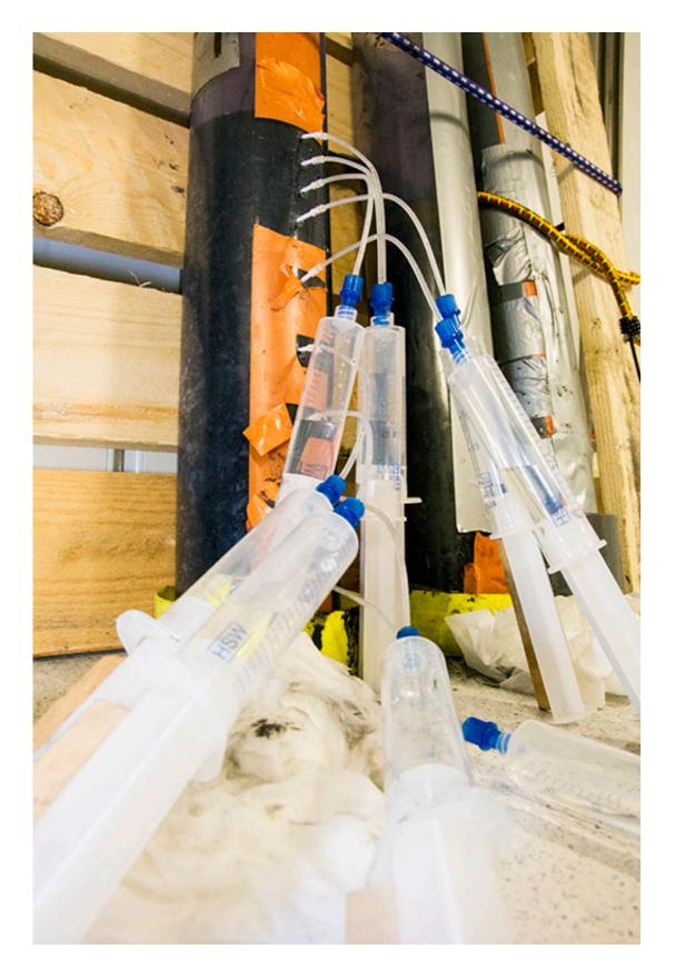
By extracting the pore water from the sediment cores, the scientist can measure
