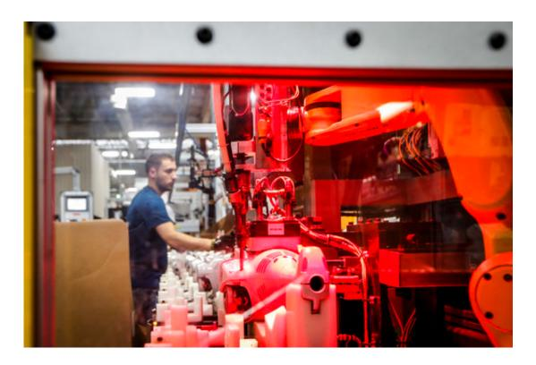
In this Thursday, May 25, 2017 photo, a collaborative robot uses a power drill to attach parts of a chainsaw body on a assembly line at Stihl Inc. production plant in Virginia Beach, Va. "The Chinese and Europeans and South Koreans are aggressively embracing robotics," says Howie Choset, a professor of robotics at Carnegie Mellon University in Pittsburgh. "We definitely are at a point where we have to keep up or get left behind." (AP Photo/John Minchillo)
