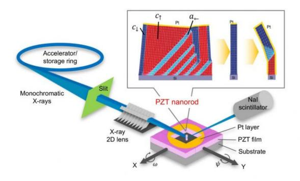
Charge screening in ferroelectric Pb(Zr,Ti)O3 nanorods was used to control their domain pattern. The c-domain fraction markedly increased with as the rod width decreased, while the a-domain formation prevailed by metallization of their sidewall. All the observed results could be explained by the depolarizing field, arising from the imperfect charge screening. This approach could be expanded to other low-dimensional nanoscale ferroelectric systems. Credit: Tomoaki Yamada
