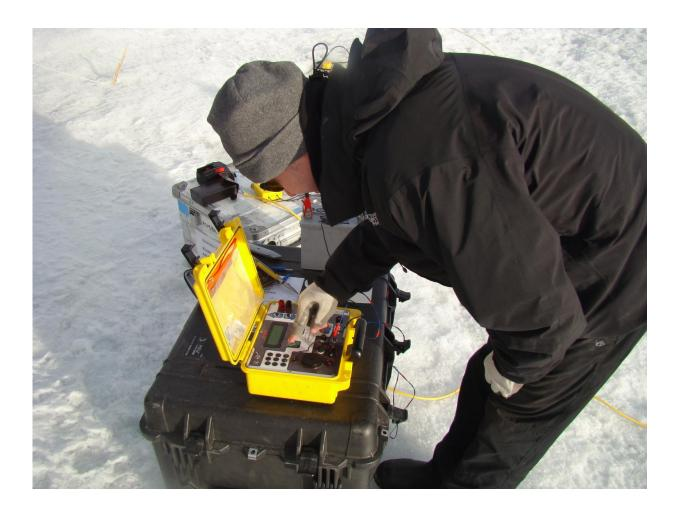
The researchers use controlled explosions to send acoustic waves through the ice, with microphones to track the data, which allows them to analyse the sediment under the ice. Credit: A D Booth
