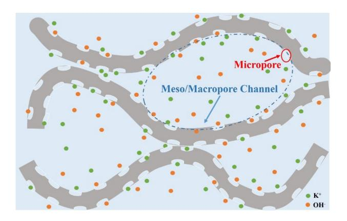
The folds of 3-D graphene make mesopore channels that work with the surface's micropores to increase the material's supercapacitive properties. Credit: Michigan Technological University
