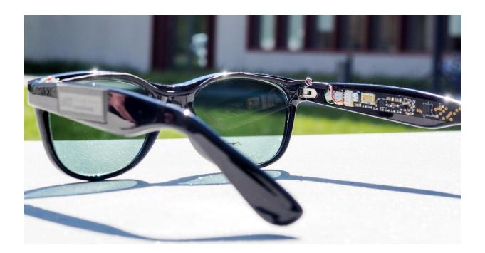
These Solar Glasses with lens-fitted semitransparent organic solar cells supply two sensors and electronics in the temples with electric power. Credit: KIT
