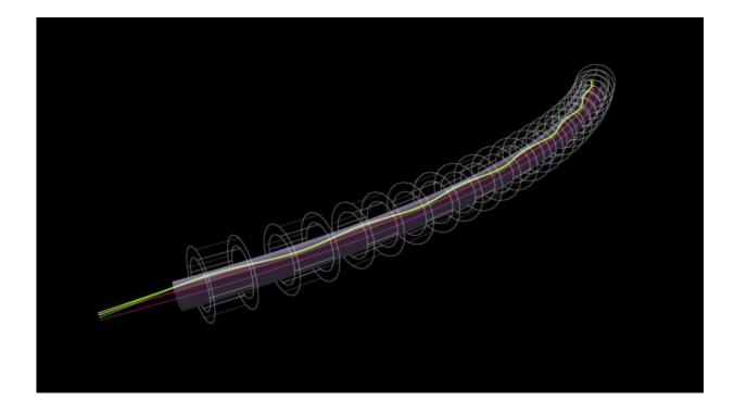
Brooks' proof-of-principle experiment showed that electron beams of five different energies could make their way through the arc of permanent magnets, each taking a somewhat different, color-coded path: dark green (18 million
