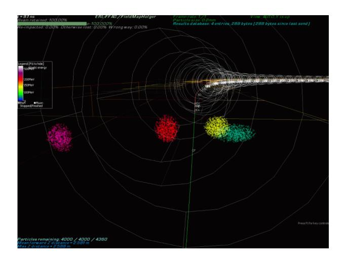
Brooks' successful test lays the foundation for the CBETA accelerator, in which bunches of electrons will be accelerated to four different energies and travel simultaneously within the same beampipe, as shown in this simulation. Credit: Brookhaven National Laboratory
