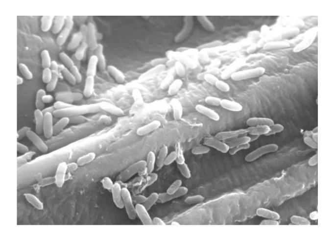
Electron microscope image of bacteria generating electricity on carbon electrode surfaces. Credit: National Institute for Materials Science (NIMS)
