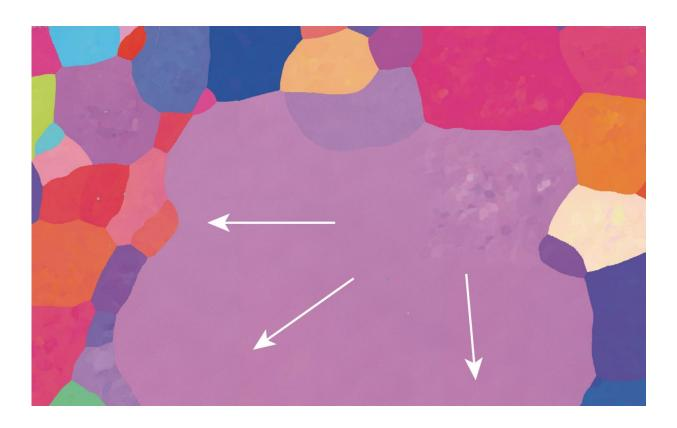
Heat treatment causing a grain to rapidly grow into a large single crystal. Credit: Toshihiro Omori (via *Nature Communications*)
