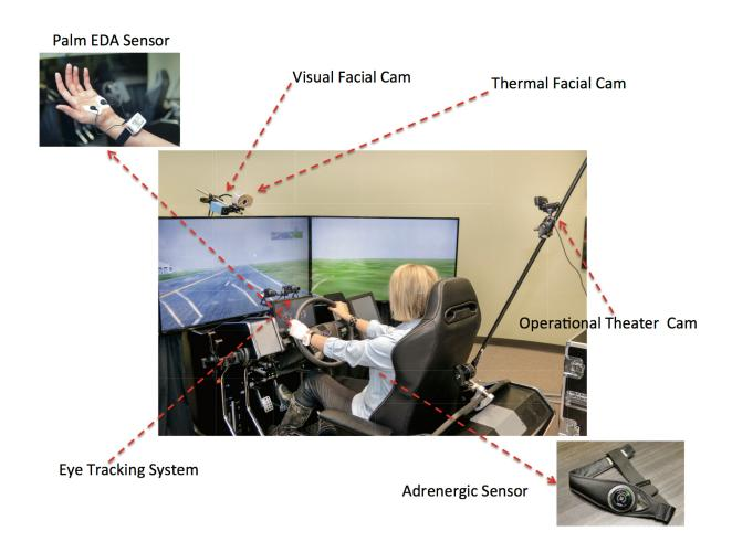
Volunteers using a driving simulator were monitored via standoff and wearable sensors, which recorded perspiration, heart rate, breathing rate, gaze and facial expressions to capture the drivers' state as they were overloaded by multitasking. Credit: University of Houston
