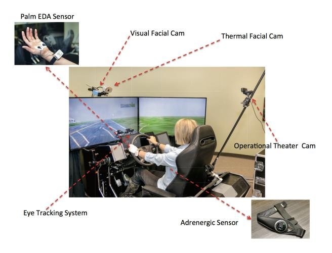
Volunteers using a driving simulator were monitored via standoff and wearable sensors, which recorded perspiration, heart rate, breathing rate, gaze and facial expressions to capture the drivers' state as they were overloaded by multitasking. Credit: University of Houston
