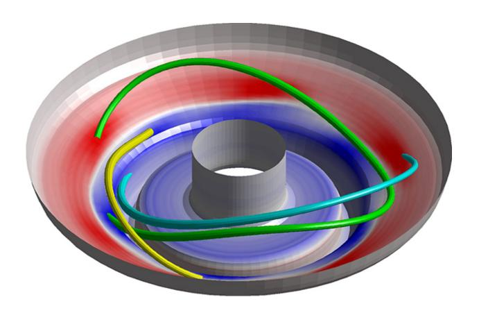
A cutaway of the lower divertor region of the National Spherical Torus Experiment in a simulation of a disruption. The red and blue colors indicate electrical "halo" currents into the walls of the tokamak. The rope-like structures show the paths of three magnetic field lines that intersect the walls. Credit: David Pfefferlé, Princeton Plasma Physics Laboratory
