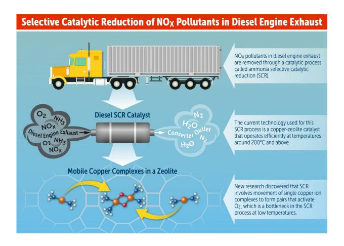
This diagram depicts a new reaction mechanism that could be used to improve catalyst designs for pollution-control systems for diesel exhaust. Credit: Purdue University /Maureen Lifton
