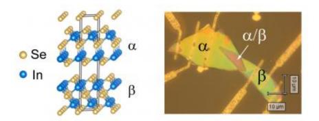
The left panel shows the schematic lattice structures of the alpha-beta In2Se3 van der Waals metal-semiconductor junction, and the right panel shows an optical micrograph of a junction device. Credit: Yi Gu
