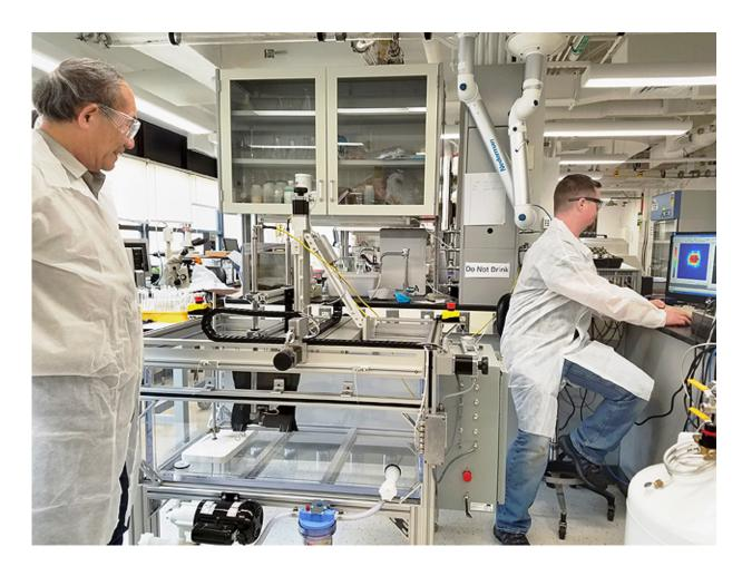
ARS engineer Cheng-Kung Liu, left, observes the airborne ultrasonic system used to scan hides for defects while ARS engineer Nick Latona, right, reviews scan images. Credit: Zerlina Muir
