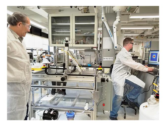
ARS engineer Cheng-Kung Liu, left, observes the airborne ultrasonic system used to scan hides for defects while ARS engineer Nick Latona, right, reviews scan images. Credit: Zerlina Muir
