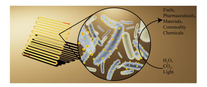
Artist's rendering of bioreactor (left) loaded with bacteria decorated with cadmium sulfide, light-absorbing nanocrystals (middle) to convert light, water and carbon dioxide into useful chemicals (right). Credit: Kelsey K. Sakimoto
