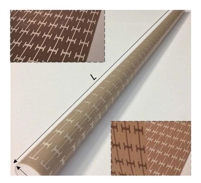
Rod shaped waveguide with two quasi-two dimensional conformal coatings that sheild the waveguide from crosstalk and blocking and allow the waveguide to be
