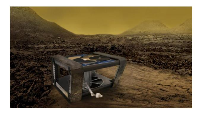
AREE is a clockwork rover inspired by mechanical computers. A JPL team is studying how this kind of rover could explore extreme environments, like the surface of Venus. Credit: NASA/JPL-Caltech
