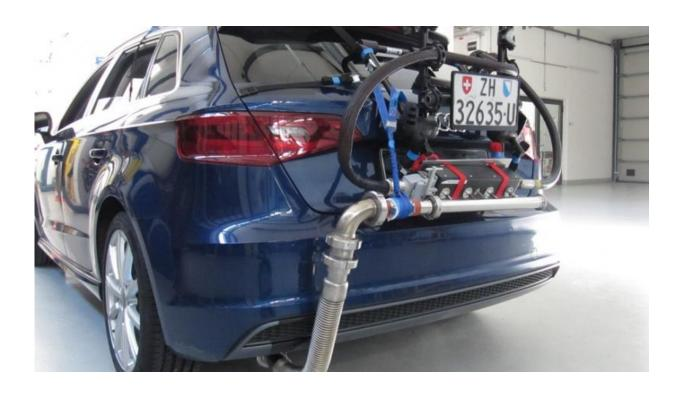
An Audi A3 with the measuring backpack to gage RDEs (real driving emissions). As of September 1, 2017, these emission measurements in actual road traffic will be mandatory for the approval of new vehicle types. Credit: Empa.
