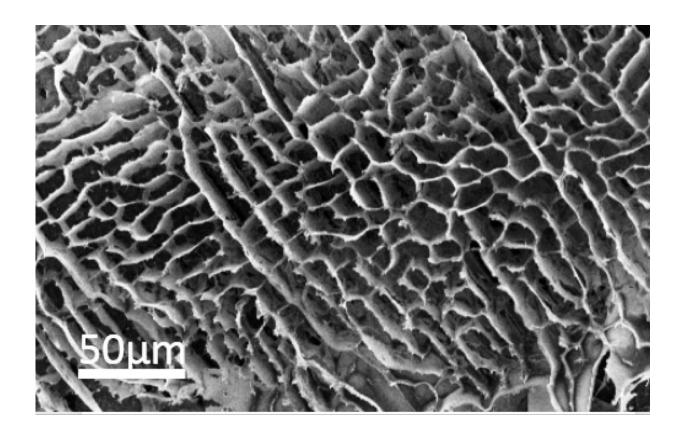
A microscope image shows the high surface area of hexagonal-boron nitride foam glued together with polyvinyl alcohol. The tough, light foam can be used to soak up carbon dioxide or as a material to shield biological tissues from lasers. Credit: Ajayan Research Group/Rice University
