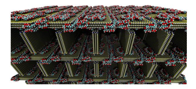
A molecular dynamics simulation shows polyvinyl alcohol molecules of carbon (teal), oxygen (red) and hydrogen (white) binding two-dimensional sheets of hexagonal-boron nitride (blue and yellow). The reusable material created at Rice University can sequester more than three times its weight in carbon dioxide. Credit: Ajayan Research Group/Rice University
