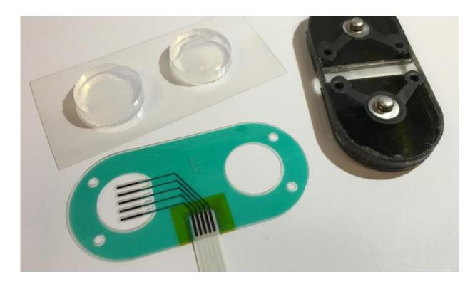
The UC study used a low electric current and carbachol gel to stimulate sweat under a sensor the size of a Band-Aid. Credit: University of Cincinnati
