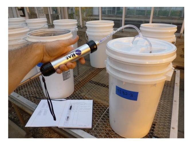
Part of the experiment, in a temperature-regulated greenhouse, measured gas release from the manure with various coverings. Credit: Brian Dougherty
