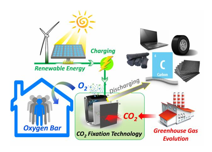
A flowchart of energy storage and carbon fixation using Li-CO2 technology. Credit: Qiao et al.
