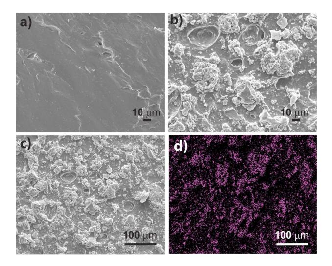
Scanning electron microscope images of (a) the chitosan film, (b) the chitosancopper metal organic framework film at 500x magnification, (c) the chitosancopper metal organic framework film at a higher magnification, and (d) an X-ray image of the film that shows the copper in pink. Credit: Reynolds Lab/Colorado State University
