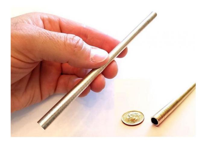
PNNL's ShAPE<sup>TM</sup> extrusion process produced this 7.5 mm diameter tube with a 0.75 mm wall thickness from flakes of a magnesium alloy. Credit: PNNL
