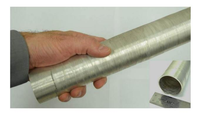
A 50 mm diameter tube with a 1.5 mm wall thickness created from a solid chunk of magnesium alloy using PNNL's ShAPE<sup>TM</sup> extrusion process. Credit: PNNL
