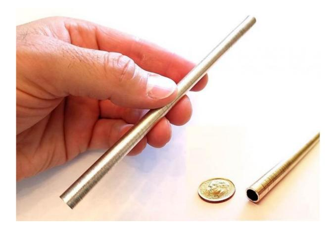
PNNL's ShAPE<sup>TM</sup> extrusion process produced this 7.5 mm diameter tube with a 0.75 mm wall thickness from flakes of a magnesium alloy. Credit: PNNL
