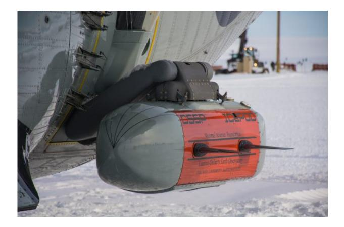
IcePod's instruments include two radars to image through the ice, lidar to measure the ice surface, cameras, and a magnetometer to better understand the bed below the ice shelf. Credit: NSF/Mike Lucibella
