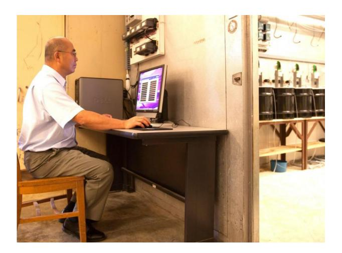
Jiqin Ni, an associate professor in Purdue's Department of Agricultural and Biological Engineering, works in his lab to develop an on-site computer and software system for agriculture-based air quality research. The system consists of commercial data acquisition hardware, a personal computer, and customdeveloped software to provide a more flexible, high-quality and user-friendly way to better understand and limit emission and pollution impact. Credit: Purdue
