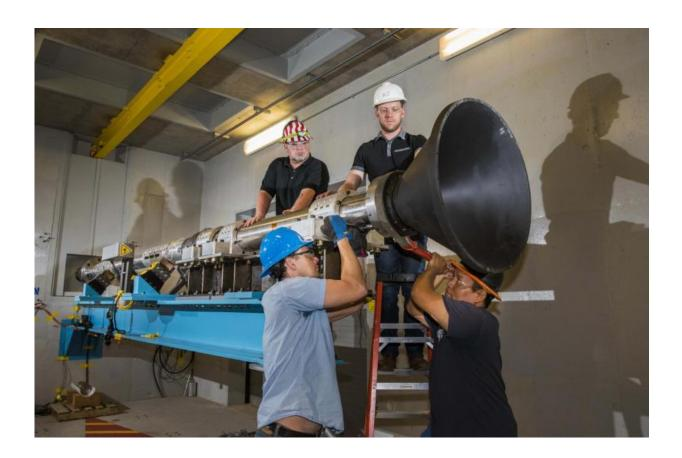
Sandia National Laboratories' Mike Beabout and Patrick Barnes, left to right top, and Mark Stroman and Jamison Lee, left to right bottom, prepare a nitrogenpowered gas gun for the labs' Alternative Pyroshock Test by installing a resonant cone to a resonant beam. Sandia successfully demonstrated a more environmentally friendly way to ensure avionics can withstand the shock from stage separation during flight. Credit: Randy Montoya
