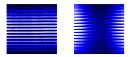
UV radiation from a relativistic electron beam is diffracted by a double-slit. In contrast to the normal light (left), the diffraction shows a deformation in the central part (right), indicating the existence of the phase singularity, which is a definite evidence of the vortex nature. Credit: Institute For Molecular Science
