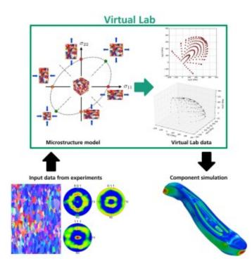
From input data obtained through experiments, via the virtual laboratory, to creation of material cards for component simulation. Credit: © Photo Fraunhofer IWM
