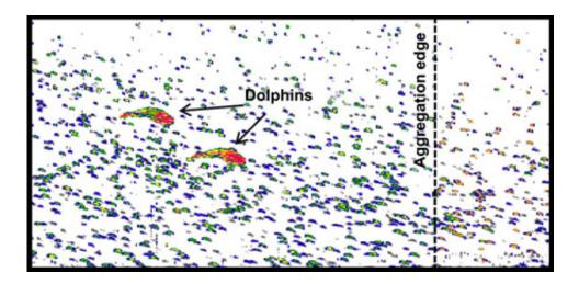
This sonar data collected by an autonomous underwater vehicle shows animals within a sound-scattering layer. The different colors indicate sound intensity and indicate two distinct aggregations or schools (likely squid to the left and fish on the right), as well as two dolphins swimming within one of the aggregations. Credit: Kelly Benoit-Bird
