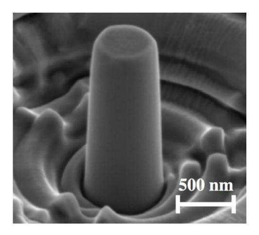
A scanning electron microscope image of one of the copper pillars used in the experiment. Credit: California Institute of Technology
