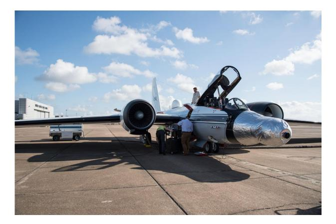
One of the WB-57F jets is readied for a test run at NASA's Johnson Space Center in Houston. The instruments are mounted under the silver casing on the nose of the plane. Credit: NASA's Johnson Space Center/Norah Moran
