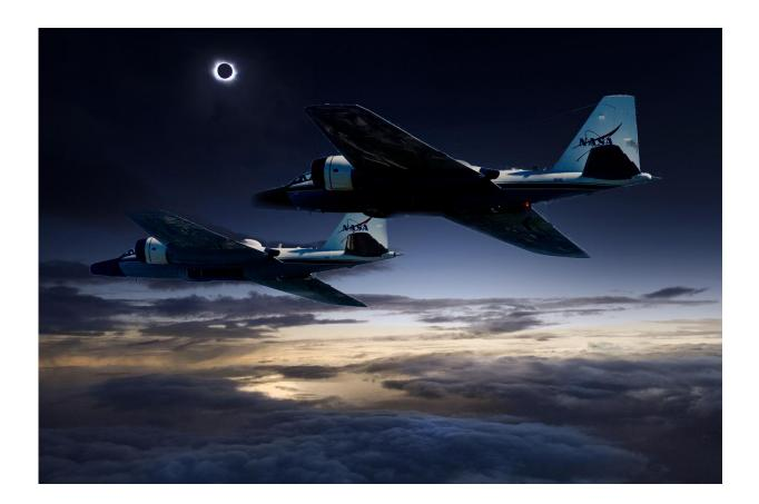
During the upcoming total solar eclipse, a team of NASA-funded scientists will observe the solar corona using stabilized telescopes aboard two of NASA's WB-57F research aircraft. This vantage point provides distinct advantages over ground-based observations, as illustrated by this composite photo of the aircraft and the 2015 total solar eclipse at the Faroe Islands. Credit: NASA/Faroe Islands/SwRI
