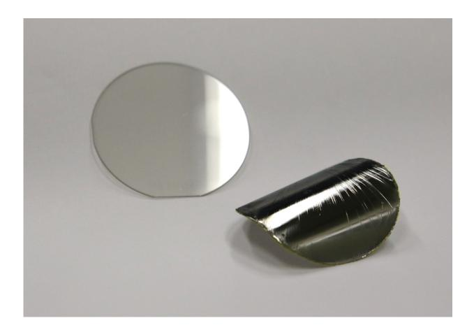
This image shows a thick bulk gallium nitride (GaN) crystal wafer (2 inches in diameter) with a GaN film in the foreground fabricated by controlled spalling (its film thickness is ~20 microns or 1/5th the thickness of a sheet of paper. Credit: Bedell/IBM Research
