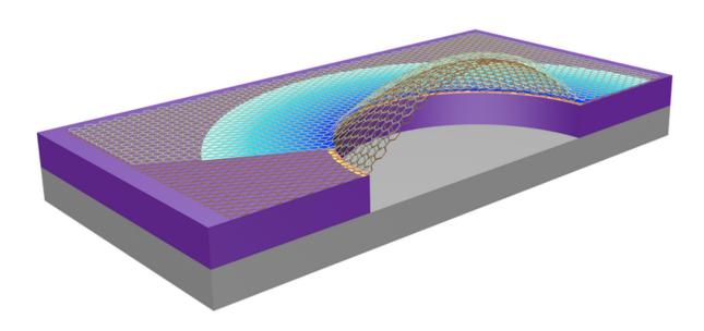
This cutaway shows the bulging that occurs when air is pumped through a hole underneath a graphene sheet. Researchers estimated the shear resistance by measuring the stretching in the sheet around the hole. The stretching for bilayer graphene (blue) is much larger than that for monolayer graphene (yellow). Credit: L. Liu, C. Weng, & G. Wang/NCNST
