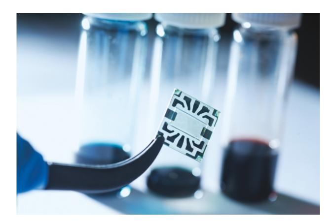
A new flexible graphene solar cell developed at MIT is seen in the transparent region at the center of this sample. Around its edges are metal contacts on which probes can be attached during tests of device performance. Credit: Stuart Darsch
