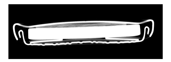
Slice from x-ray computed tomography image of a supercapacitor coin cell assembled with the electrode materials. The thin layers -- just below the coin cell lid -- are layers of electrode materials and a separator. Credit: William Kuykendall
