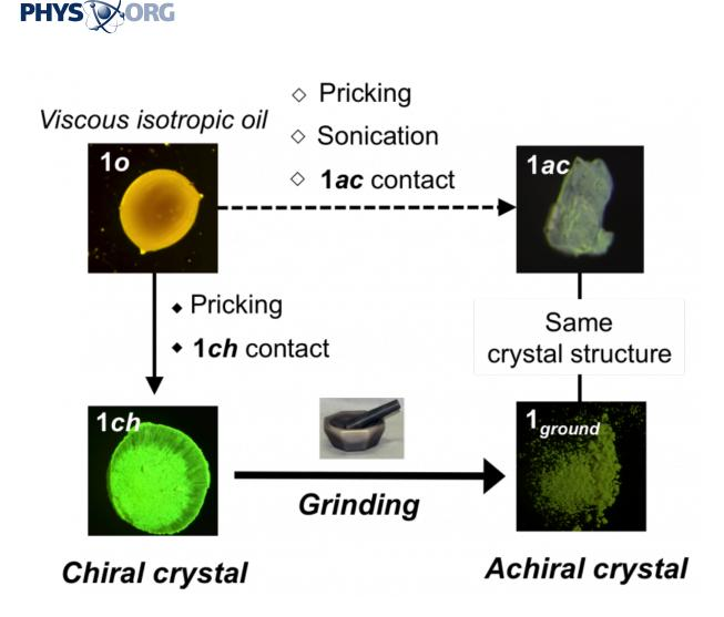
Viscous oil made from gold and isocyanide crystalizes in response to stimuli either into a chiral crystal or achiral crystal. A chiral crystal turns to an achiral crystal when ground. Phase transitions cause color changes. Credit: Jin M. et al., Journal of the American Chemical Society, May 23, 2017
