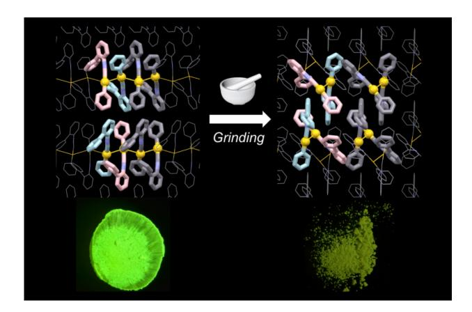
Grinding chiral crystals of gold and isocyanide complexes caused them to transition into achiral crystals while simultaneously changing their emission properties. Credit: Hokkaido University
