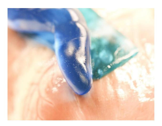
A new, flexible adhesive material inspired by the glue secreted by slugs adheres to biological tissues (even when wet) without causing toxicity, and can be formed into either sheets (teal blue) or custom shapes (dark blue) Credit: Wyss Institute at Harvard University
